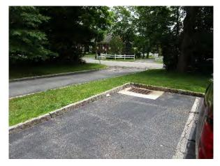
A rain garden can be installed north of the building to capture, treat, and infiltrate stormwater runoff from the roof and parking lot. Parking spaces near the catch basin in the rear parking lot can be converted to porous pavement to capture and infiltrate stormwater runoff from the parking lot. A preliminary soil assessment suggests that the soils have suitable drainage characteristics for green infrastructure.
