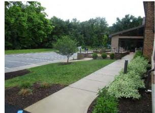
A rain garden can be installed southwest of the building to capture, treat, and infiltrate the stormwater coming from the top of the building. Pervious pavement can be installed in the southeastern corner of the parking lot to capture stormwater runoff from the parking lot. A preliminary soil assessment suggests that the soils have suitable drainage characteristics for green infrastructure.
