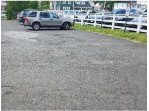
Parking spaces in the parking lot to the north of the building can be converted to porous pavement to capture and infiltrate stormwater runoff from the parking lot. On the north side of the building downspout planter boxes can be installed to help capture stormwater runoff from the building's roof. A preliminary soil assessment suggests that more soil testing would be required before determining the soil's suitability for green infrastructure.
