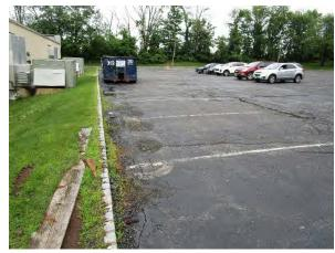
Pervious pavement can be installed in both parking lots to capture and infiltrate stormwater runoff from the parking lot. Bioretention systems can be installed in the turfgrass areas by using curb cuts to direct water from the pavement into them. A preliminary soil assessment suggests that more soil testing would be required before determining the soil's suitability for green infrastructure.
