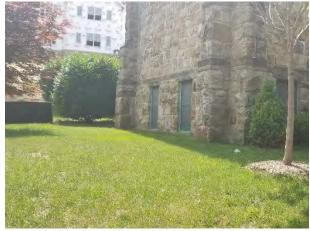
A rain garden can be installed along the southeast side of the church and at the bottom of a hill on the property to capture, treat, and infiltrate parking lot and rooftop runoff. A preliminary soil assessment suggests that more soil testing would be required before determining the soil's suitability for green infrastructure.
