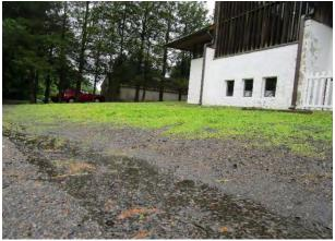
A rain garden can be installed to capture, treat, and filter runoff from the rooftop of the easternmost building on the property. Pervious pavement can be installed in the parking spaces to infiltrate the water from the driveway, and downspout planter boxes can be installed along the front of the school. A preliminary soil assessment suggests that the soils have suitable drainage characteristics for green infrastructure.
