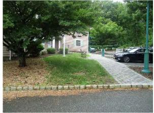
Pervious pavement can be installed in the parking spaces west of the building to capture and infiltrate stormwater. A rain garden can be installed to the northwest of the building to capture, treat, and infiltrate stormwater runoff from the roof. A preliminary soil assessment suggests that the soils have suitable drainage characteristics for green infrastructure.
