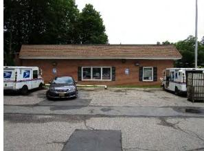
Parking spaces in the parking lot to the east of the building can be converted to porous pavement to capture and infiltrate stormwater runoff from the parking lot and the downspout. A septic system in the turfgrass area north of the building limits rain garden opportunities. A preliminary soil assessment suggests that the soils have suitable drainage characteristics for green infrastructure.
