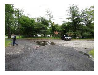
Parking spaces in the parking lot to the south of the building can be converted to porous pavement to capture and infiltrate stormwater runoff from the roof via the downspouts, which are disconnected. A preliminary soil assessment suggests that more soil testing would be required before determining the soil's suitability for green infrastructure.
