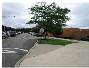
Parking spaces in the parking lot to the southeast of the building can be converted to pervious pavement to capture and infiltrate stormwater runoff from the parking lot. Additional parking spaces throughout the site could be retrofitted as well. A small bioretention system can be installed adjacent to the shed to manage the rooftop runoff. A preliminary soil assessment suggests that the soils have suitable drainage characteristics for green infrastructure.
