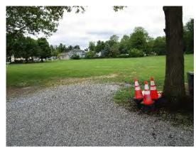
A rain garden can be installed to the west of the building nearby the baseball field. A preliminary soil assessment suggests that the soils have suitable drainage characteristics for green infrastructure.
