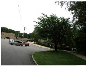
Pervious pavement can be installed in the center parking spaces to capture and infiltrate stormwater runoff from the parking lot. A stormwater planter can be installed by depaving a portion of the wide sidewalk. A curb cut can be used to intercept stormwater runoff from the parking lot. A preliminary soil assessment suggests that the soils have suitable drainage characteristics for green infrastructure.
