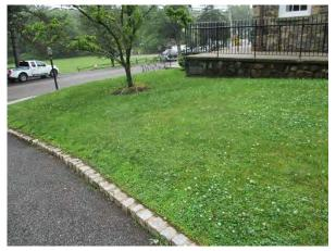
Bioretention systems can be installed on the southeast and southwest side of the building to capture, treat, and infiltrate rooftop runoff. To help with stormwater capture, downspout planter boxes can be placed along the southwestern part of the building. A preliminary soil assessment suggests that the soils have suitable drainage characteristics for green infrastructure.
