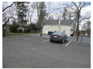
Parking spaces in the parking lot to the west of the building can be converted to porous pavement to capture and infiltrate stormwater runoff from the parking lot. Two rain gardens can be installed in the turfgrass area near the entrance of the building and a third in the rear of the building to capture more runoff from the parking lot. A preliminary soil assessment suggests that more soil testing would be required before determining the soil's suitability for green infrastructure.
