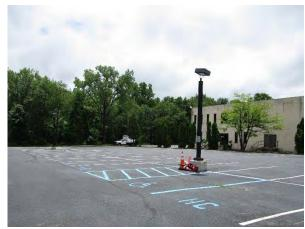
Parking spaces at the southeast end of the parking lot can be converted to pervious pavement to capture and infiltrate stormwater from the parking lot. A preliminary soil assessment suggests that the soils have suitable drainage characteristics for green infrastructure.
