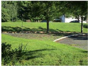
Two sections of parking spaces can be converted to pervious pavement to capture and infiltrate parking lot runoff. Sections of turfgrass adjacent to the parking lot can be converted to rain gardens to capture, treat, and infiltrate parking lot runoff. A preliminary soil assessment suggests that more soil testing would be required before determining the soil's suitability for green infrastructure.
