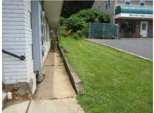
A rain garden can be installed between the post office and the parking lot to capture, treat, and infiltrate rooftop runoff since no gutters are installed. A preliminary soil assessment suggests that more soil testing would be required before determining the soil's suitability for green infrastructure.
