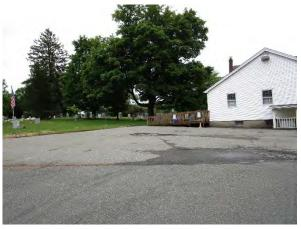
Pervious pavement can be installed south of the building near two disconnected downspouts to capture and infiltrate stormwater runoff from the parking lot and building. Parking spaces in the north parking lot can also be retrofitted with pervious pavement. A preliminary soil assessment suggests that the soils have suitable drainage characteristics for green infrastructure.
