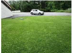
Parking spaces in the parking lot to the southwest of the building can be converted to pervious pavement to capture and infiltrate stormwater runoff from the parking lot. A rain garden can be installed in the turfgrass area west of the building to capture, treat, and infiltrate stormwater runoff from the roof. A preliminary soil assessment suggests that the soils have suitable drainage characteristics for green infrastructure.
