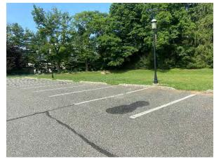
Rain gardens can be installed to the northwest of the parking lot and to the southeast of the building to capture, treat, and infiltrate the stormwater runoff from the parking lot and building rooftop. This will require curb cuts and downspout redirection beneath the sidewalk. A preliminary soil assessment suggests that the soils have suitable drainage characteristics for green infrastructure.
