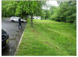
A rain garden can be installed to reduce the flooding that occurs east of the parking lot. Pervious pavement can be installed in the parking lot row directly west of the building to capture stormwater runoff from both the parking lot and the rooftop. A preliminary soil assessment suggests that more soil testing would be required before determining the soil's suitability for green infrastructure.
